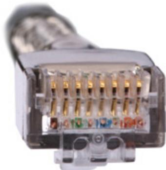
**Step 2** Hold an RJ45 connector and turn it 45°. Observe the top edges of the metal contact strips. **Figure 11-30** shows an unqualified piece.
