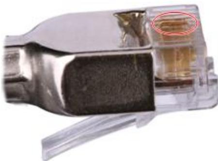
**Step 3** Check whether the contact strips are clean. If they are not clean and the dirt cannot be removed, replace it with a new RJ45 connector. **Figure 11-31** shows an unqualified piece.
