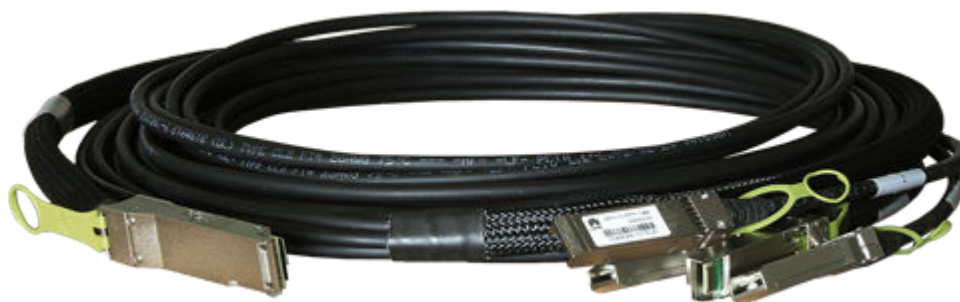
Figure 6-40 Appearance of a QSFP+ to 4*SFP+ or QSFP28 to 4*SFP28 high-speed cable
