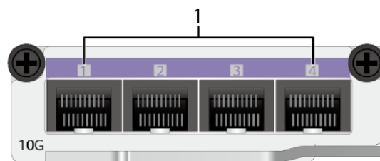
Figure 8-7 Indicators on the ES5D000X4S01
