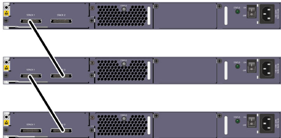
Figure 8-94 Chain topology of a stack
