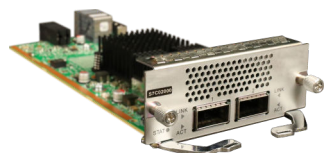
Figure 8-87 Appearance of the S7C02000
