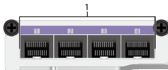
Figure 8-14 Ports on the ES5D00G4SA01
