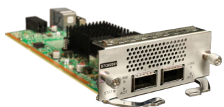
Figure 8-81 Appearance of the S7Q02001
