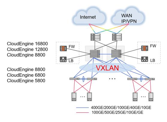
Note: VXLAN can also be used on campus networks to support flexible service deployment in different service areas.
