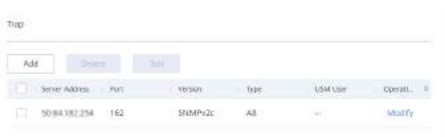
Figure 5-24 Trap server address management area
