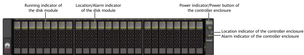
Figure 3-59 Indicators on the front panel of a 2 U 25-disk controller enclosure
