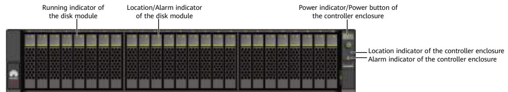
Figure 3-25 Indicators on the front panel of a 2 U 25-disk controller enclosure
