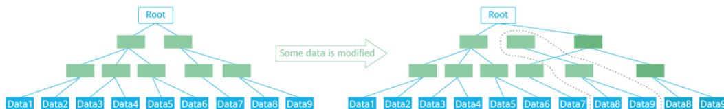
OceanStor Dorado uses the redirect-on-write (ROW) mechanism to create snapshots for file systems. ROW allows the file system to write newly created or modified data to a new space instead of overwriting the original data, ensuring high reliability and scalability of the file system. With ROW, file system snapshots can be created in seconds and do not occupy additional space unless the source files are deleted or modified.
