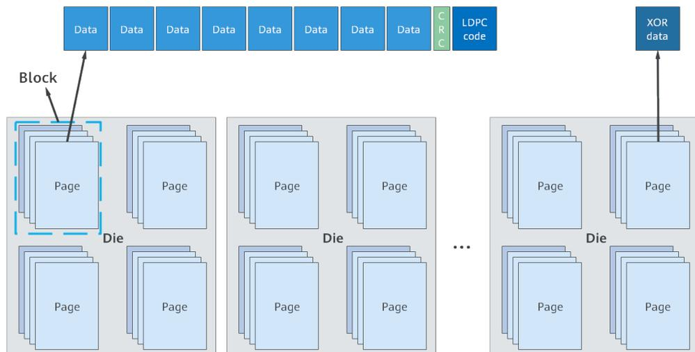
LDPC uses linear codes defined by the check matrix to check and correct errors. When data is written to pages on the NAND flash, the system calculates the LDPC verification information and writes it to the pages with the user data. When data is read from the pages, LDPC verifies and corrects the data.
