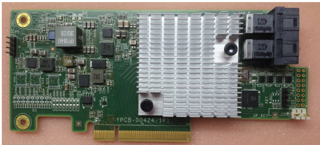
Figure 2-1 SAS3008 SAS Controller Card
