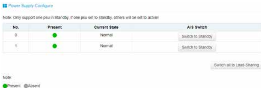
Figure 44 PSU Active Standby
