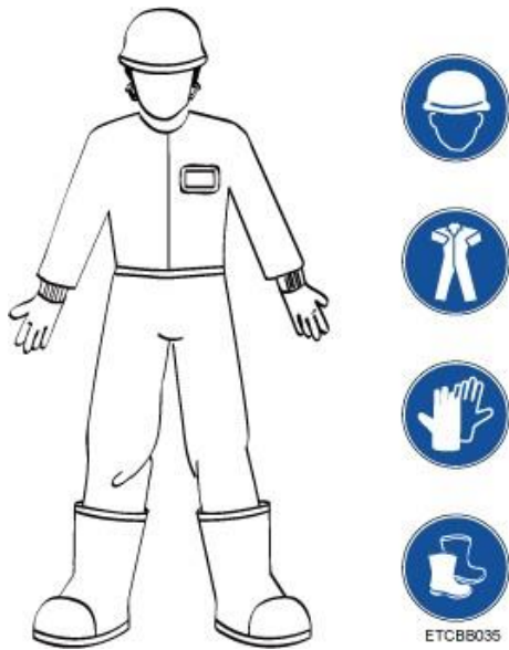
Figure 8-1 Safety Protection Measures
